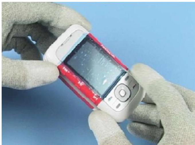
3. Open the E-COVER Assembly. Remove the battery if it is still inserted.
