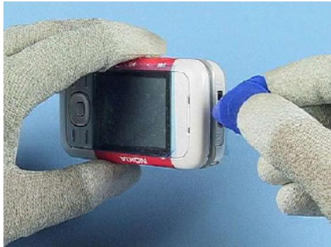
5. Use the SRT-6 only in direction shown. Do not shift the SRT-6 along the side where the keys are located.
