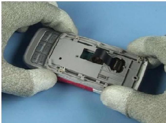
4. Push the connector into position shown.
