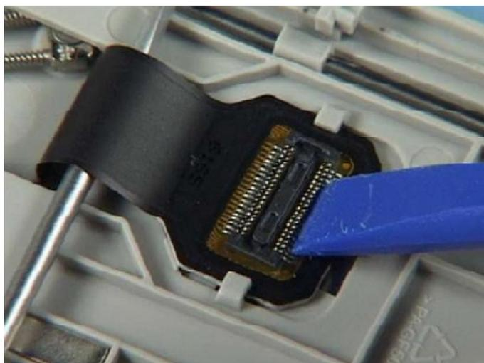
26. After disassembling the upper part the SIDE FLEX can be removed easily.
