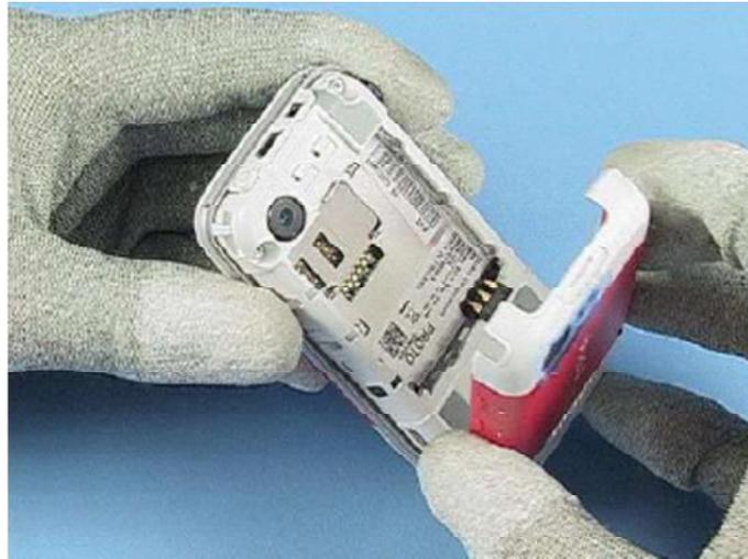
4. Use the SRT-6 to pry open the A-COVER assembly.
