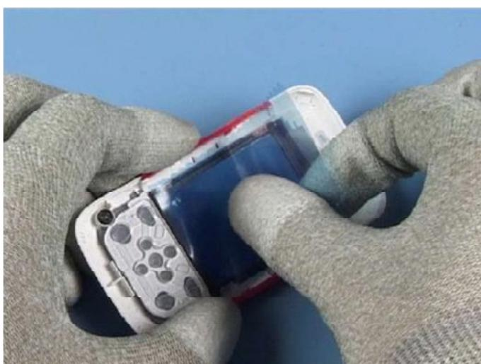
9. Release and remove the FUNCTIONAL KEYMAT.
