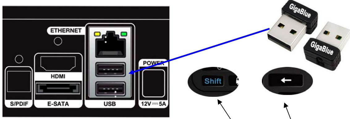
Then please pairing them, the method is that please press "SHIFT" and "BACKSPACE" button at same time, and the remote should close to USB within 3mm, one of LED on keyboard side will flash during
