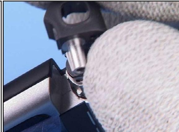
16. Remove the HINGE CAP RIGHT and then the Push to Open Button.
