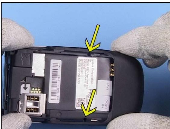
8. Hold the assembly as shown. Locate the 2 holes in the D-COVER.
