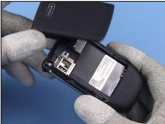
3. Remove the battery, SIM,  $\mu$ SD card if still inside.
