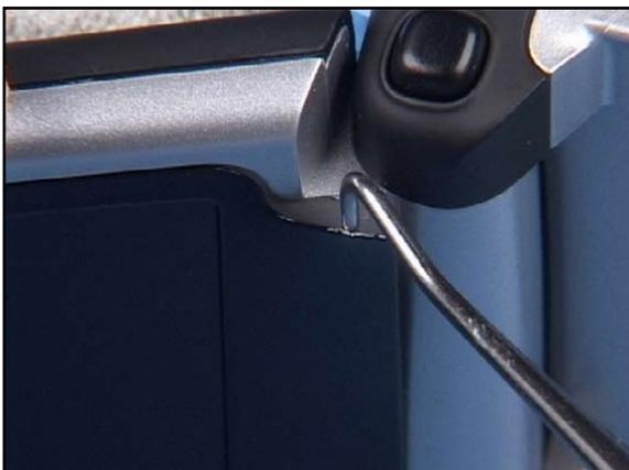
5. Carefully lift up the lower side of the DISPLAY BEZEL, first with the dental tool.
