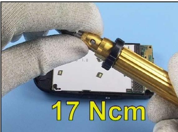
11. Set the correct torque and tighten in.
