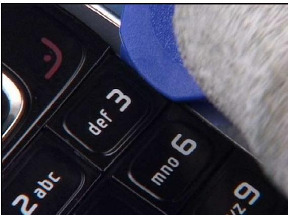
5. Carefully pry open the KEYMAT with SRT-6 at key 3.
