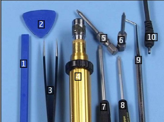
1. Needed tools: 1. SS-93, 2. SRT-6, Metal tweezers, 4. Torque driver, 5. Torx plus size 5 bit, 6. Torx plus size 6 bit, 7. Torx plus driver size 6, 8. Torx plus driver size 5, 9. Dental pick and 10. DC-Plug.
