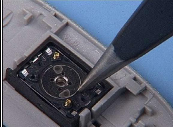
2. Ensure that the dust net is glued on the Earpiece, then place the EARPIECE evenly into the Gasket.
