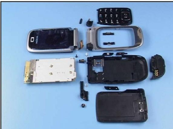
27. The disassembly procedure is now complete.
