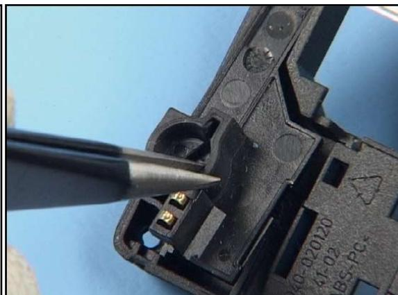
24. Remove the BLUETOOTH ANTENNA with tweezers.
