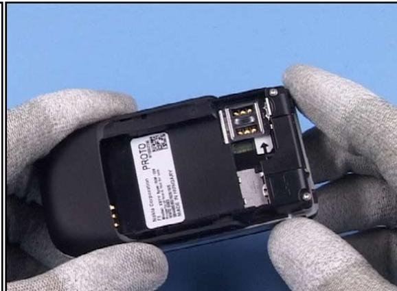
4. Check that there is no SIM or SD card still inserted before continuing.
