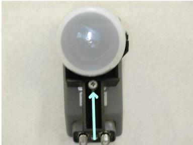
Align the **CENTER** of LNB Holder Unit at the R10 marking of LNB Guide.
