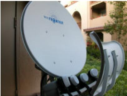
**TIP:** Assemble and align Toroidal at ground level with small TV and receiver right next to you. This will save you a tremendous time. (If you have a sat finder equipment, maybe not.) After the alignment, you can put the assembled dish on your roof and adjust azimuth only, take a minute and reducing the risk and sweat!
