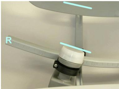
After inserting LNB Holder Unit into guide, loosely tight screw so that the unit can stay on the guide. You will tighten this screw at the very end of this process. You will find that surface of LNB and Sub Reflectors are symmetrically aligned.
