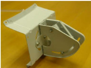
There are 3 connection points on Back Mount Tilt unit. Use B8 on the center with B13. Use Phillips driver to tighten. Then, tighten B4 with B14 with hands. Nuts should be on the back the unit so you can adjust skew angle later on.
